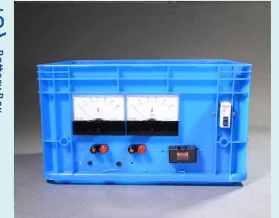
The battery box is designed to make the test table more compact and easy to monitor and protect the battery.
